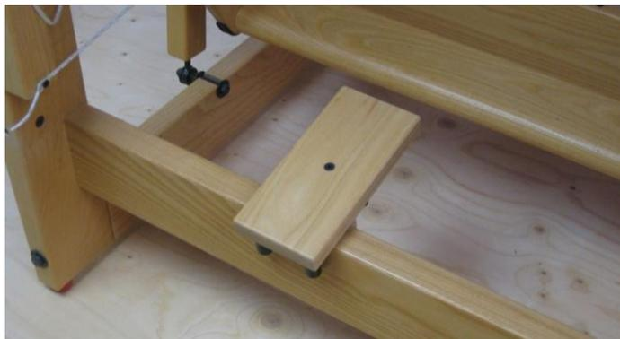
Is the block positioned correctly, tighten the black knurled nuts on the back of the sensor block.
