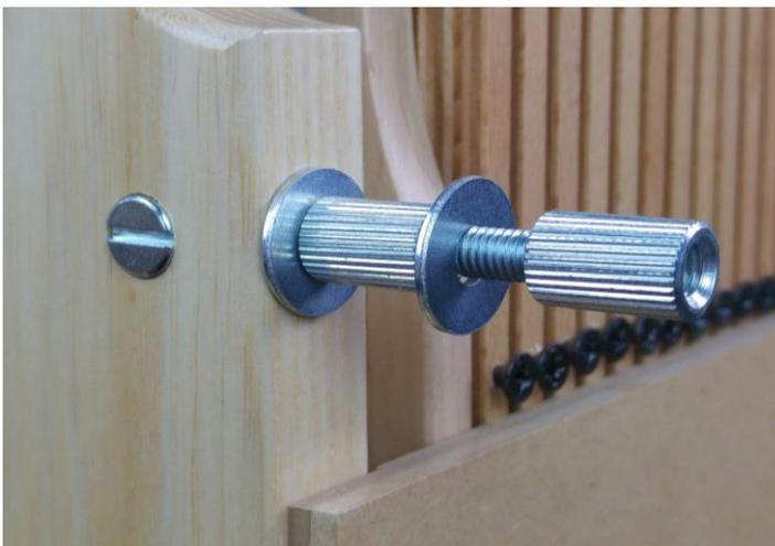
Slip on a washer, screw a knurled nut on and tighten it firmly onto the washer and place a second washer onto the end.
