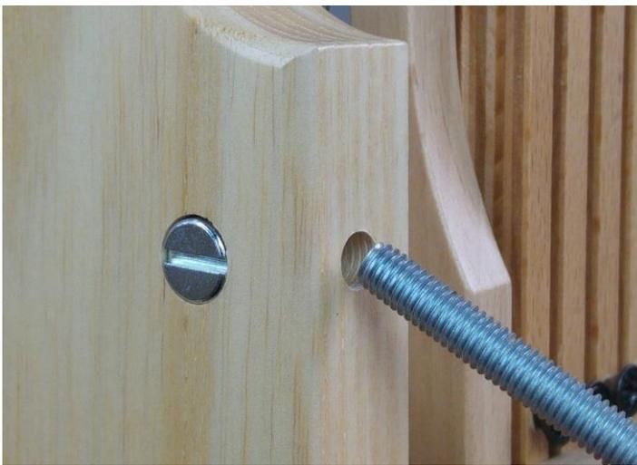
Insert the threaded rod into the hole and screw it into the barrel nut. Turn the end by hand until it sits tight.
