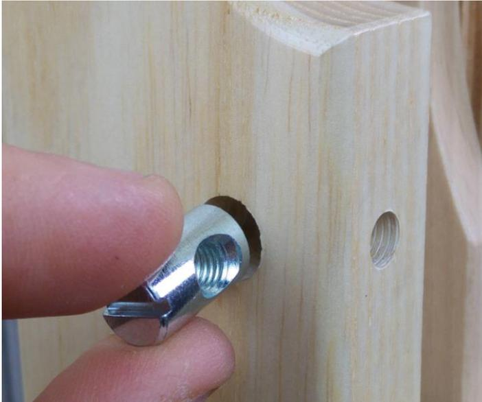
Insert the barrel nut into the hole in the side of the middle section. The slots indicate the direction of the threaded hole in the nuts. Make sure these slots are facing outwards.
