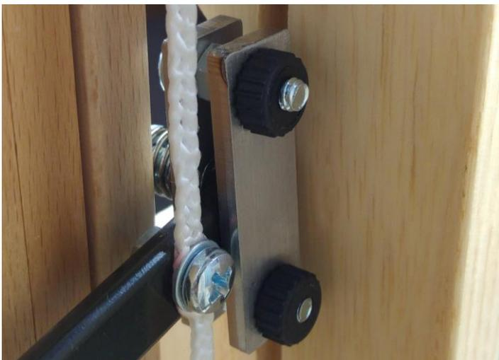
Don't tighten the knurled nuts too much. You want to be able to move the block around until it is properly aligned with the dobbie top sensor – after the dobbie is attached.
