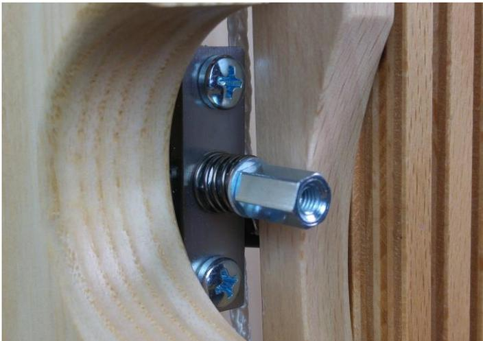
Mount the switch block onto the knife (the slanted metal strip that takes the activated dobbie hooks down) on the front side of the loom, as shown. The switch block should be facing the dobbie unit.
