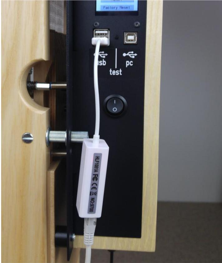
Put the USB to Ethernet adapter in one of the USB ports.
