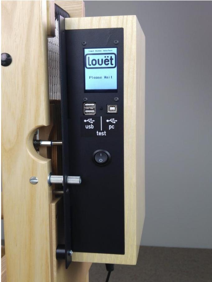
First make sure the Dobby 2.0 is switched off by checking the power switch on the front. Connect the Dobby 2.0 with the cable from the power supply. After that connect the power supply to the main power supply. The flat side of the connector should face the wooden case of the doobby.
