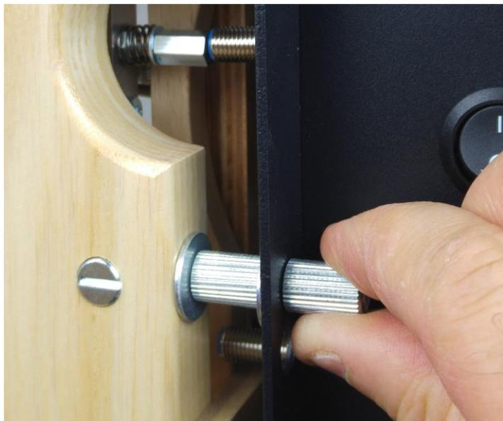
Slide the Dobby 2.0 over the threaded ends, and fasten it with the second knurled nut on each end.
